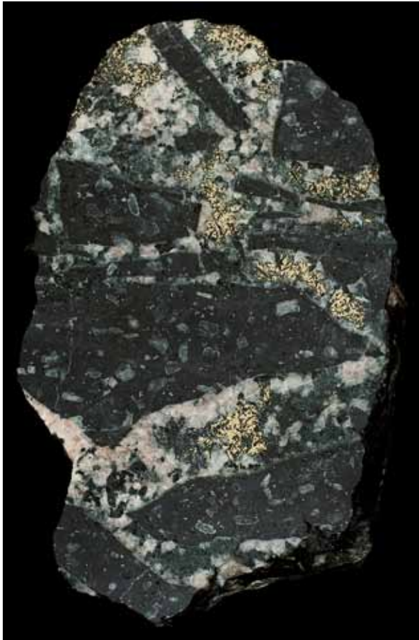
Fig. 4. Volcanic clasts, cemented by quartz veins with K-feldspar and chalcopyrite. Bedovina mine. The maximum length of the sample is 11cm.
