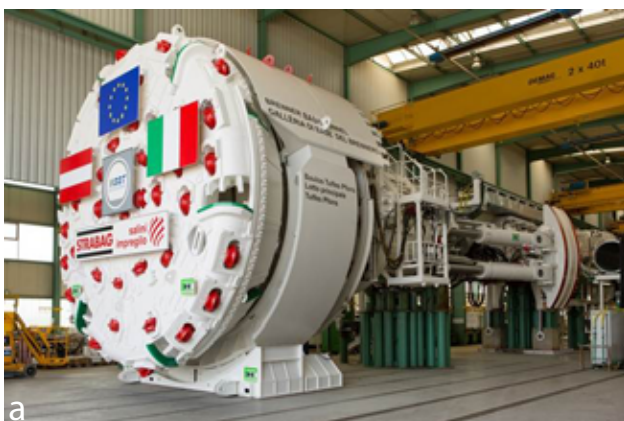
Fig. 12: The tunnel boring machine (TBM). a) The open gripper TBM. Approximately 70 % of the BBT is being built using mechanical excavation. b) The TBM will excavate 15 km of the exploratory tunnel in south direction.
