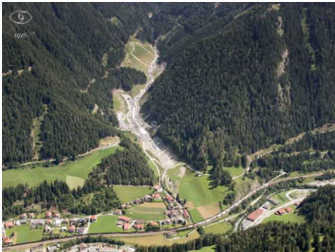
Fig. 6: Overview of the Padaster valley. a) Current view of the Padaster valley and of the village of Siegreith: The construction (bulk tunnel, diversion tunnel) is completed; the depositing of excavated material is in progress. b) After the deposition of excavated material is completed the Padaster valley will be fully recultivated (reforestation, new stream course, ecological compensation areas, etc.).
