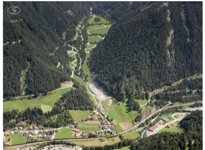
Fig. 6: Overview of the Padaster valley. a) Current view of the Padaster valley and of the village of Siegreith: The construction (bulk tunnel, diversion tunnel) is completed; the depositing of excavated material is in progress. b) After the deposition of excavated material is completed the Padaster valley will be fully recultivated (reforestation, new stream course, ecological compensation areas, etc.).
